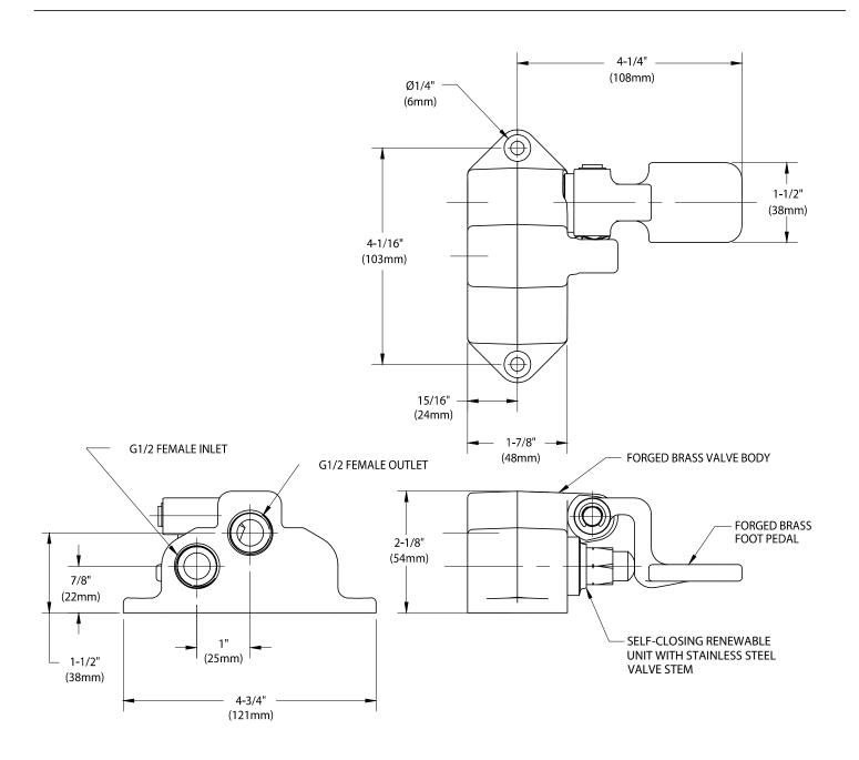
NOTE: 1. FIXTURE IS FULLY ASSEMBLED AND FACTORY
