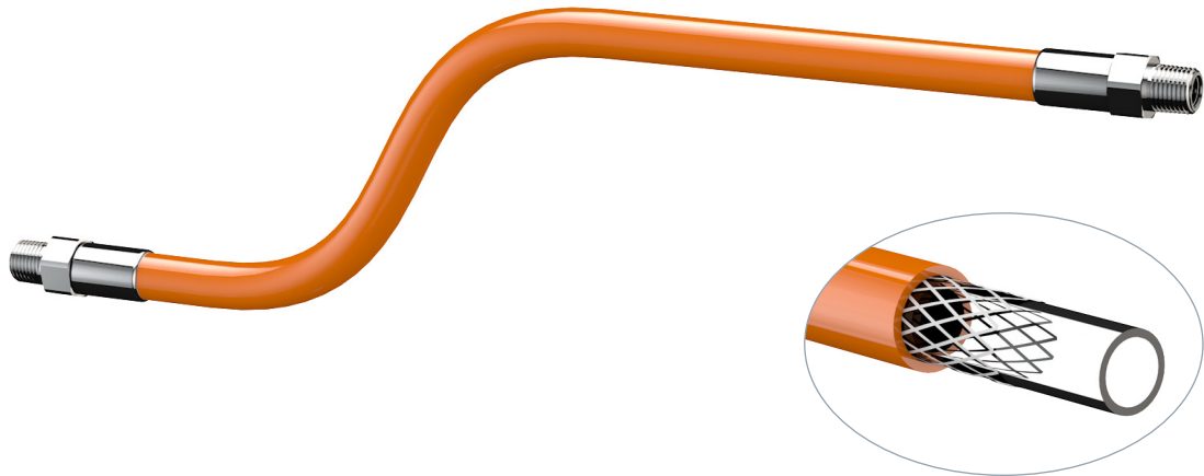
Reinforced PVC hose with nylon braid and PVC inner core
