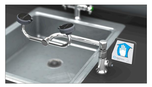
**Application:** Eye/face wash for mounting on counter next to sink. Spray heads swivel 90 degrees from storage to operational position. Water flow is activated by flag handle.
