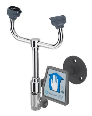
**Application:** Eyewash for wall mounting. Two GS-Plus™ spray-type spray heads deliver a flood of water for rinsing eyes. Unit is provided without bowl or drain for waste water. Note: Floor drain should be provided underneath unit to prevent accumulation of water on floor.
