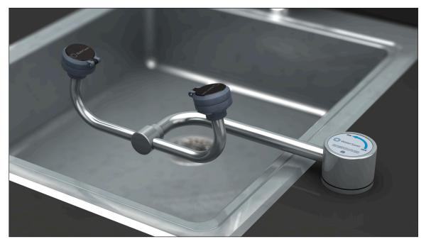
**Application:** All-stainless steel AutoFlow<sup>™</sup> eyewash for mounting on counter next to sink. Unit is constructed entirely in stainless steel. Ideal for use in highly corrosive environments, cleanrooms and pharmaceutical applications. Swinging the spray head assembly horizontally out over the sink activates the water flow. The unit remains in operation until the spray head assembly is swung back into the storage position, closing the valve.
