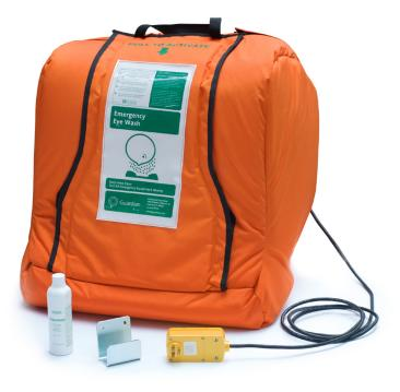
**Preparation:** Top operate unit, fill unit with clean potable water and add bacteriostatic additive (supplied with unit). Additive protects against growth of bacteria, fungus, algae and acanthamoeba. Unit should be inspected regularly and water in unit should be changed at least once every six months.
