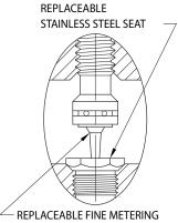
REPLACEABLE FINE METERING STAINLESS STEEL FLOATING NEEDLE
