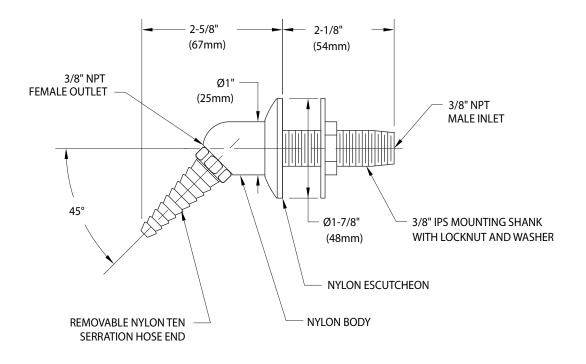
NOTE: FITTING IS COLOR-CODED PER SERVICE INDEX COLOR AS STANDARD.
