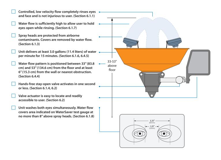
Location: Install eye/face wash unit within 10 seconds (approximately 55 feet) of hazard, on the same level as hazard and with unobstructed travel path. Where strong acids or caustics are being handled, emergency eye/face wash units should be located adjacent to the hazard, and an appropriate professional should be consulted for advice on the proper distance. (Section 6.4.2; B5)
