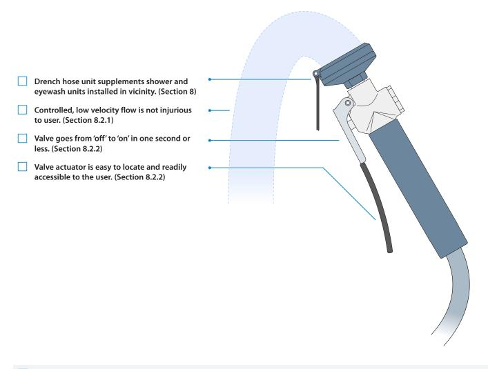
Location: Install drench hose unit in area free of debris or obstructions. (Section 8.2.3.2)
