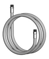
AP350-100-096 8 ft. reinforced PVC hose for eyewash/ drench hose and drench hose unts. 3/8" NPT male swivel inlet, 3/8" NPT male outlet.
