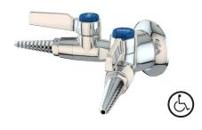
Mounting: For installation on vertical surfaces (such as drywall) where there is no access behind wall during installation. Flange is threaded onto nipple stubbed out of wall. Threaded escutcheon is then backed up to wall to secure valve and conceal pipe.
