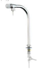
**Application:** Recirculating deck mounted faucet for distilled, deionized or reverse osmosis water. Faucet is fully recirculating to eliminate all "dead legs" in pure water system.
