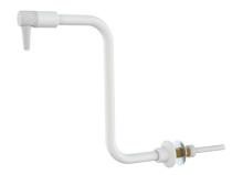
Application: Panel mounted polypropylene-lined gooseneck for distilled, deionized and reverse osmosis water. Fitting has exterior brass casing and interior lining of inert polypropylene. Pure water comes in contact only with inert plastic.
