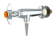
**Mounting:** For installation on vertical surfaces (such as pipe chases and service carriers) where there is access behind surface during installation. Threaded mounting shank is inserted through hole in surface and secured with locknut and washer.
