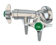
Mounting: For installation on vertical surfaces (such as drywall) where there is no access behind wall during installation. Wye fitting is threaded onto nipple stubbed out of wall. Threaded escutcheon is then backed up to wall to secure fixture and conceal pipe.
