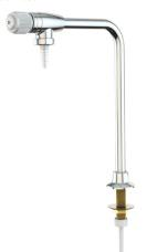
**Application:** Deck mounted faucet for distilled, deionized or reverse osmosis water. Faucet has exterior brass casing and interior lining of inert polypropylene. Pure water comes in contact only with inert plastic.
