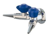
Mounting: For installation on vertical surfaces (such as drywall) where there is no access behind wall during installation. Wye fitting is threaded onto nipple stubbed out of wall. Threaded escutcheon is then backed up to wall to secure valve and conceal pipe.
