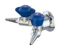
Mounting: For installation on vertical surfaces (such as drywall) where there is no access behind wall during installation. Wye fitting is threaded onto nipple stubbed out of wall. Threaded escutcheon is then backed up to wall to secure valve and conceal pipe.
