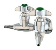
Mounting: For installation on vertical surfaces (such as drywall) where there is no access behind wall during installation. Wye fitting is threaded onto nipple stubbed out of wall. Threaded escutcheon is then backed up to wall to secure fixture and conceal pipe.
