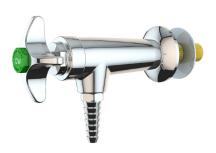
Mounting: For installation on vertical or horizontal surfaces (such as pipe chases and service carriers) where there is access behind surface during installation. Threaded mounting shank is inserted through hole in surface and secured with locknut and washer.
