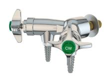
Mounting: For installation on vertical or horizontal surfaces (such as pipe chases and service carriers) where there is access behind surface during installation. Threaded mounting shank is inserted through hole in surface and secured with locknut and washer.
