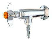
Mounting: For installation on vertical surfaces (such as drywall) where there is no access behind wall during installation. Valve is threaded onto nipple stubbed out of wall. Threaded escutcheon is then backed up to wall to secure valve and conceal pipe.
