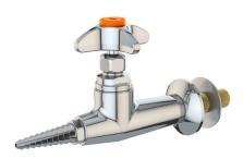
Mounting: For installation on vertical or horizontal surfaces (such as pipe chases and service carriers) where there is access behind surface during installation. Threaded mounting shank is inserted through hole in surface and secured with locknut and washer.
