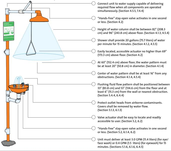
LOCATION Install safety station within 10 seconds (approximately 55 feet) of hazard, on the same level as
