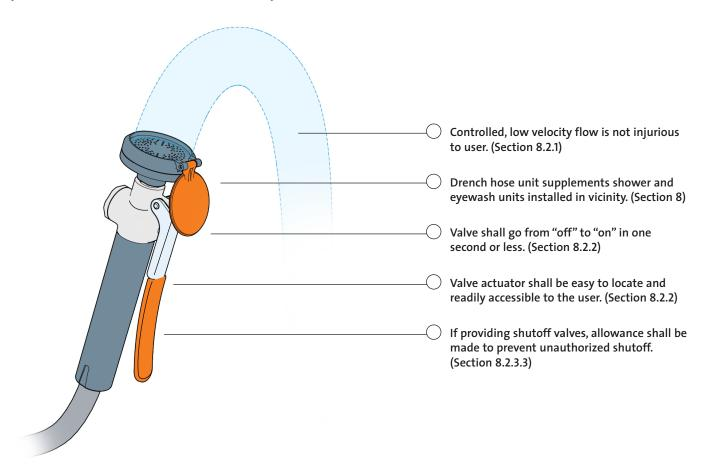
LOCATION Install drench hose unit in area free of debris or obstructions. (Section 8.2.3.2)
