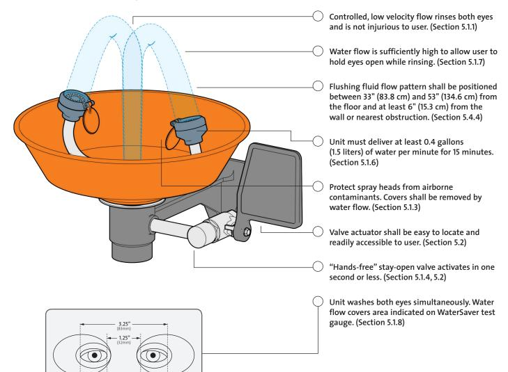
Install eyewash wash unit within 10 seconds (approximately 55 feet) of hazard, on the same level LOCATION
