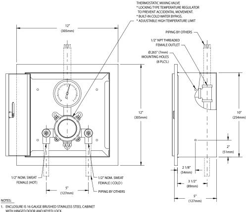
WITH HINGED DOOR AND KEYED LOCK. 2. MIXING VALVE IS CERTIFIED BY CSA TO MEET ASSE 1071 AND
