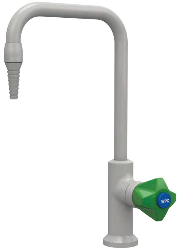
Components are polished and buffed, then plated with one layer of nickel and one layer of chrome in WaterSaver's environmentally-controlled process. Following plating, components are powder coated with LabGuard clear powder coating applied over the chrome plated surface.
