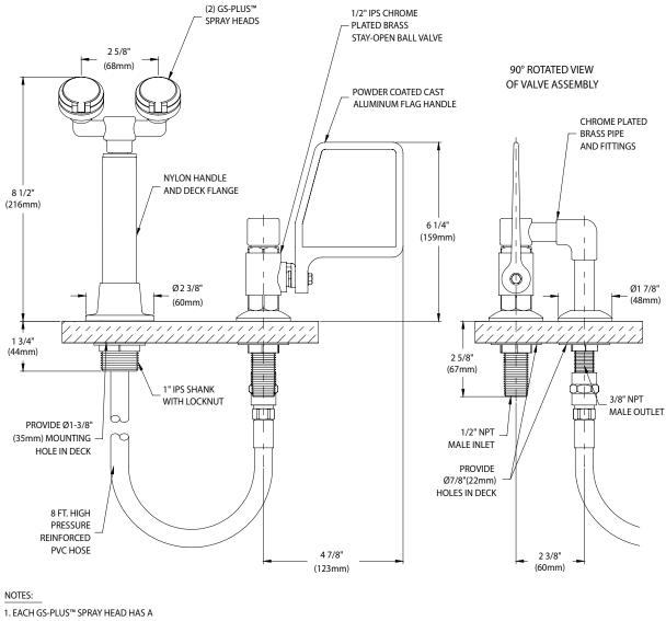
1. EACH GS-PLUS™ SPRAY HEAD HAS A "FLIP-TOP" DUST COVER, INTERNAL FLOW CONTROL AND FILTER TO REMOVE IMPURITIES FROM THE WATER FLOW. 2. HOSE SHOULD NOT BE USED IN APPLICATIONS WHERE WATER PRESSURE EXCEEDS 90 PSI. HOSE SHOULD BE INSPECTED PERIODICALLY FOR DETERIORATION.
