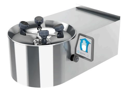
**Application:** Barrier-Free WideArea<sup>™</sup> eye/face wash for wall mounting. Bowl is lowered and extended to permit access by wheelchair user. Profile of unit is "flattened" to comply with maximum height and knee clearance requirements. Unit has stainless steel bowl and wrap-around skirt to conceal valve, drain and piping.
