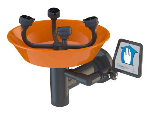
**Application:** WideArea<sup>™</sup> eye/face wash for wall mounting. Constructed entirely in PVC and PVC-coated brass. Ideal for use in industrial environments where harsh acids or caustics are present. Four GS-Plus<sup>™</sup> spray-type outlet heads deliver a flood of water over a wide area of coverage for complete rinsing of eyes and face.
