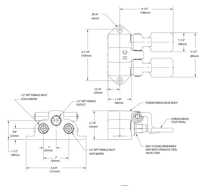
NOTES: 1. FIXTURE IS FULLY ASSEMBLED AND FACTORY TESTED PRIOR TO SHIPMENT. 2. FIXTURE HAS POLISHED CHROME PLATED FINISH.
