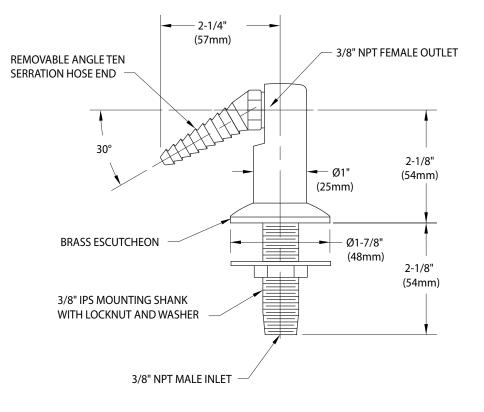
NOTE: FITTING IS FURNISHED WITH A POWDER-COATED FINISH COLOR-CODED PER SERVICE INDEX COLOR AS STANDARD. OTHER FINISHES ARE AVAILABLE UPON REQUEST.
