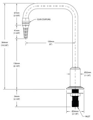
**Inlet:** Furnished with G1/2 mounting shank, locknut and washer. Available with choice of inlet connections (see below).
