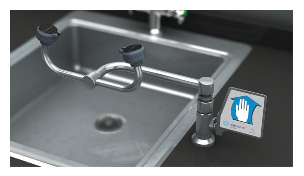
**Application:** All-stainless steel eyewash for mounting on counter next to sink. Unit is constructed entirely in stainless steel. Ideal for use in highly corrosive environments, cleanrooms and pharmaceutical applications. Spray heads swivel 90 degrees from storage to operational position. Water flow is activated by flag handle.
