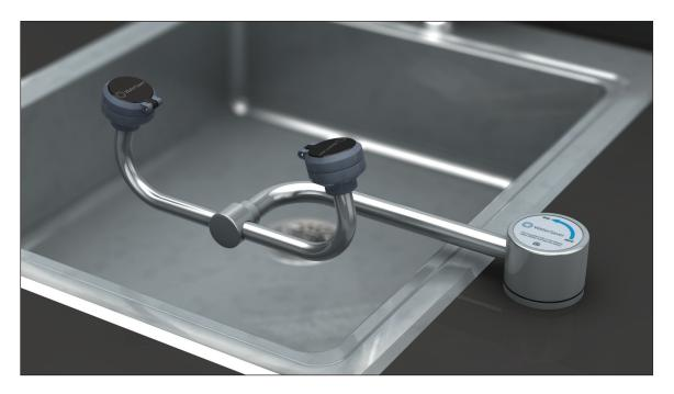
**Application:** All-stainless steel AutoFlow™ eyewash for mounting on counter next to sink. Unit is constructed entirely in stainless steel. Ideal for use in highly corrosive environments, cleanrooms and pharmaceutical applications. Swinging the spray head assembly horizontally out over the sink activates the water flow. The unit remains in operation until the spray head assembly is swung back into the storage position, closing the valve.
