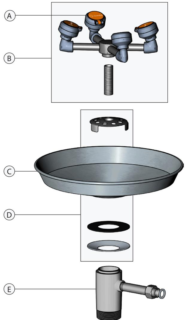
Safety stations are designed for easy assembly in the field. Essentially, these units are assembled from the "bottom up", as described below:
