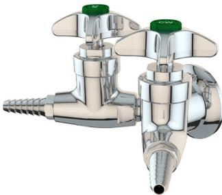
**Mounting:** For installation on vertical surfaces (such as drywall) where there is no access behind wall during installation. Wye fitting is threaded onto nipple stubbed out of wall. Threaded escutcheon is then backed up to wall to secure fixture and conceal pipe.
