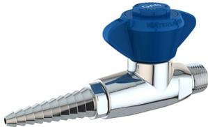
**Application:** On/off control of all laboratory gases at pressures up to 100 PSI. Valve has spring loaded handle that locks in closed position. To open valve, handle must be lifted up to unlock. Valve is certified for natural gas service by CSA International.
