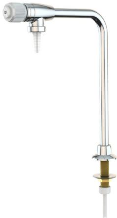
**Application:** Deck mounted faucet for distilled, deionized or reverse osmosis water. Faucet has exterior brass casing and interior lining of inert polypropylene. Pure water comes in contact only with inert plastic.
