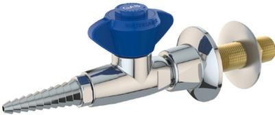
**Mounting:** For installation on vertical or horizontal surfaces (such as pipe chases and service carriers) where there is access behind surface during installation. Threaded mounting shank is inserted through hole in surface and secured with locknut and washer.
