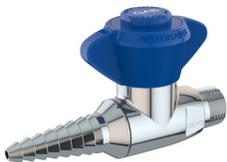
**Application:** On/off control of all laboratory gases at pressures up to 100 PSI. Valve has spring loaded handle that locks in closed position. To open valve, handle must be lifted up to unlock. Valve is certified for natural gas service by CSA International.
