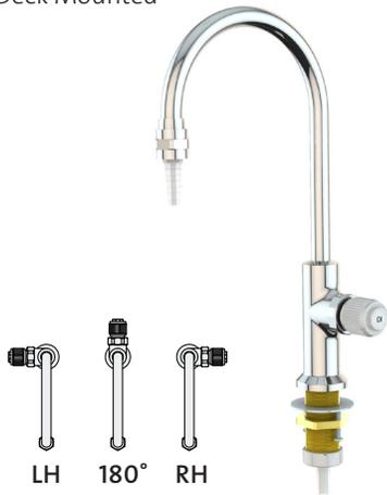
**Application:** Deck mounted faucet for distilled, deionized or reverse osmosis water. Faucet has exterior brass casing and interior lining of inert polypropylene. Pure water comes in contact only with inert plastic.
