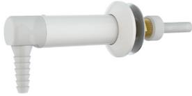
**Application:** Panel mounted polypropylene-lined outlet fitting for distilled, deionized and reverse osmosis water. Fitting has exterior brass casing and interior lining of inert polypropylene. Pure water comes in contact only with inert plastic.
