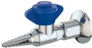
**Mounting:** For installation on vertical surfaces (such as drywall) where there is no access behind wall during installation. Flange is threaded onto nipple stubbed out of wall. Threaded escutcheon is then backed up to wall to secure valve and conceal pipe.
