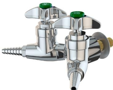
**Mounting:** For installation on vertical or horizontal surfaces (such as pipe chases and service carriers) where there is no access behind surface during installation. Threaded mounting shank is inserted through hole in surface and secured with locknut and washer.
