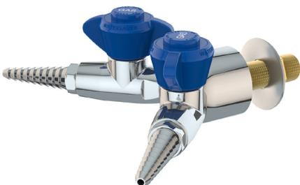
**Mounting:** For installation on vertical or horizontal surfaces (such as pipe chases and service carriers) where there is access behind surface during installation. Threaded mounting shank is inserted through hole in surface and secured with locknut and washer.
