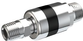
**BO191-2M Quick Connect Fitting:** Body has internal shut-off valve. Polished chrome plated finish. 3/8" NPT male inlet, 1/4" NPT male outlet.
