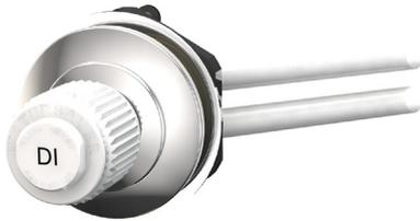
**Application:** Panel mounted fume hood valve for distilled, deionized or reverse osmosis water. Valve is designed for angle face hood. Valve has exterior brass casing and interior lining of inert polypropylene. Pure water comes in contact only with inert plastic.
