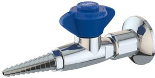
**Mounting:** For installation on vertical surfaces (such as drywall) where there is no access behind wall during installation. Flange is threaded onto nipple stubbed out of wall. Threaded escutcheon is then backed up to wall to secure valve and conceal pipe.
