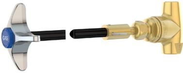
**Application:** Rod-type straight pattern valve for installation within side wall or underneath deck of hood. Valve inlet and outlet are at 180 degrees. Furnished complete with anodized aluminum extension rod, guide plate and handle.
