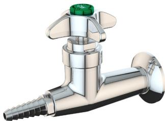
**Mounting:** For installation on vertical surfaces (such as drywall) where there is no access behind wall during installation. Valve is threaded onto nipple stubbed out of wall. Threaded escutcheon is then backed up to wall to secure valve and conceal pipe.
