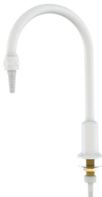
**Application:** Deck mounted polypropylene-lined gooseneck for distilled, deionized and reverse osmosis water. Fitting has exterior brass casing and interior lining of inert polypropylene. Pure water comes in contact only with inert plastic.
