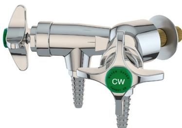
**Mounting:** For installation on vertical or horizontal surfaces (such as pipe chases and service carriers) where there is no access behind surface during installation. Threaded mounting shank is inserted through hole in surface and secured with locknut and washer.
