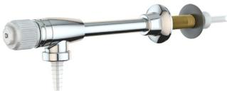
**Application:** Panel mounted faucet for distilled, deionized or reverse osmosis water. Faucet has exterior brass casing and interior lining of inert polypropylene. Pure water comes in contact only with inert plastic.
