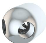
**BI141:** Panel mounted wye fitting. 3/8" NPT female inlet, (2) 3/8" NPT female outlets at 90 degrees.
