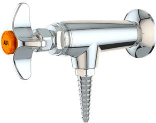
**Mounting:** For installation on vertical surfaces (such as drywall) where there is no access behind wall during installation. Valve is threaded onto nipple stubbed out of wall. Threaded escutcheon is then backed up to wall to secure valve and conceal pipe.
