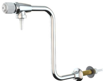
**Application:** Panel mounted faucet for distilled, deionized or reverse osmosis water. Faucet has exterior brass casing and interior lining of inert polypropylene. Pure water comes in contact only with inert plastic.
