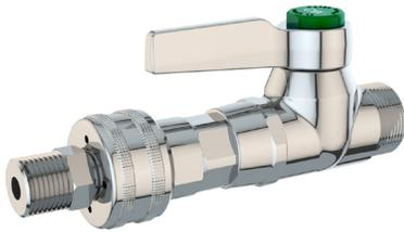
**Application:** High flow water valve for use on process and chilled water systems. Valve is used for supply and return connections. Ball valve design provides high capacity and minimizes pressure drop through valve.
