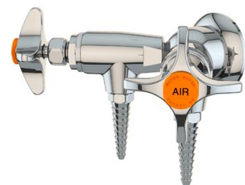
**Mounting:** For installation on vertical surfaces (such as drywall) where there is no access behind wall during installation. Wye fitting is threaded onto nipple stubbed out of wall. Threaded escutcheon is then backed up to wall to secure fixture and conceal pipe.
