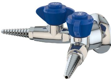
**Mounting:** For installation on vertical surfaces (such as drywall) where there is no access behind wall during installation. Wye fitting is threaded onto nipple stubbed out of wall. Threaded escutcheon is then backed up to wall to secure valve and conceal pipe.
