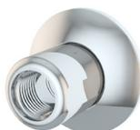
**BI158FT:** Panel mounted flange with adjustable escutcheon. 3/8" NPT female inlet and outlet. Furnished with threaded escutcheon.
