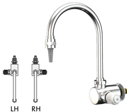
**Application:** Panel mounted faucet for distilled, deionized or reverse osmosis water. Faucet has exterior brass casing and interior lining of inert polypropylene. Pure water comes in contact only with inert plastic.
