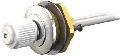
**Application:** Panel mounted fume hood valve for distilled, deionized or reverse osmosis water. Valve is designed for straight face hood. Valve has exterior brass casing and interior lining of inert polypropylene. Pure water comes in contact only with inert plastic.
