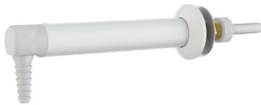
**Application:** Panel mounted polypropylene-lined outlet fitting for distilled, deionized and reverse osmosis water. Fitting has exterior brass casing and interior lining of inert polypropylene. Pure water comes in contact only with inert plastic.
