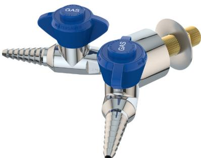
**Mounting:** For installation on vertical or horizontal surfaces (such as pipe chases and service carriers) where there is access behind surface during installation. Threaded mounting shank is inserted through hole in surface and secured with locknut and washer.
