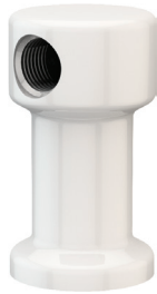
BI231VR Turret base. 3/8" NPT female inlet, single 3/8" NPT female outlet.
