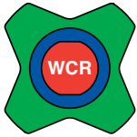
Coolant Water Return
